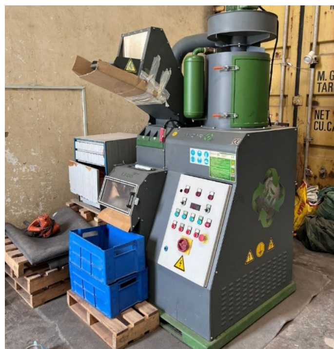
Figure 19: Cable granulator at Enviroserve
