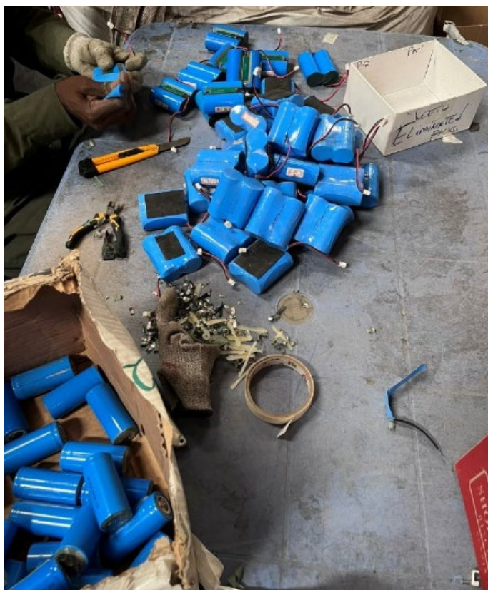
Figure 20: Dismantling of Battery Packs at Enviroserve
